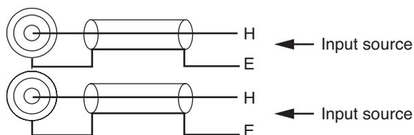
Upper and lower RCA inputs are internally, passively mixed.
