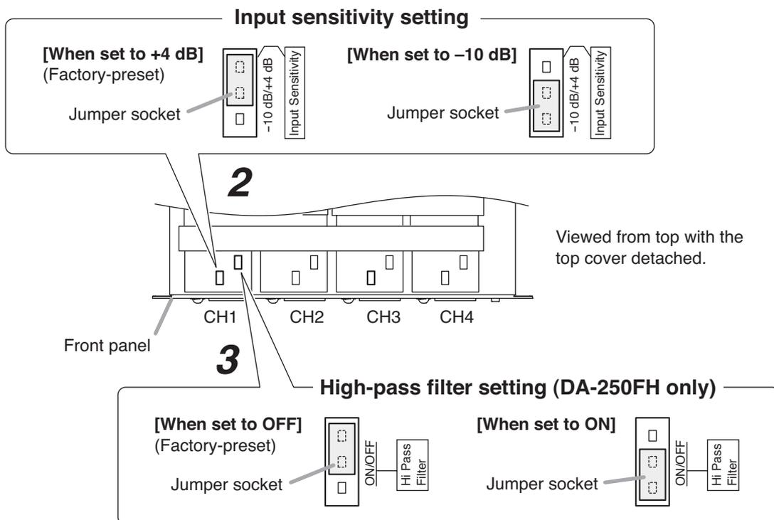
**Step 4.** Change the jumper socket position to "ON" or "OFF" for the High-pass filter as illustrated above. (DA-250FH only)
