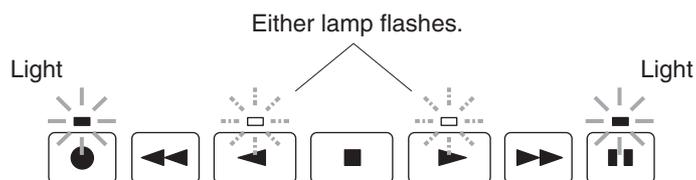
**Step 5.** Press the Pause button [■] or the flashing Play button [◀] or [▶]. The tape will begin to record, and the Direction indicator lamp will light to indicate the current tape direction.
