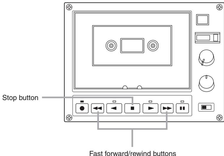
**Step 1.** Press the double arrow [◀◀/▶▶] button pointing to the direction that the tape is moving during recording or playback to fast-forward the tape. Pressing the double arrow button pointing to the opposite direction will rewind the tape.
