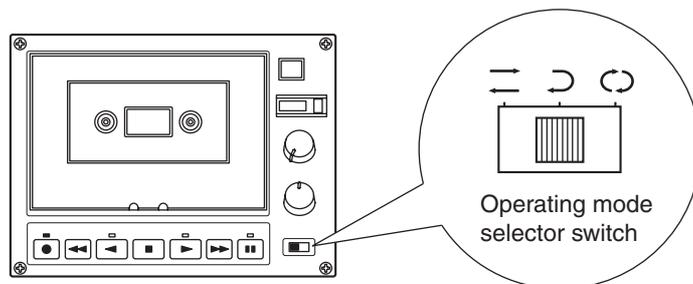
The following table shows tape operation when the Operating mode selector switch and other buttons are pressed.
