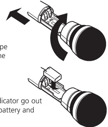
**Note:** Should the Red battery status Led Indicator go out during operation, this indicates a flattened battery and should be changed .
