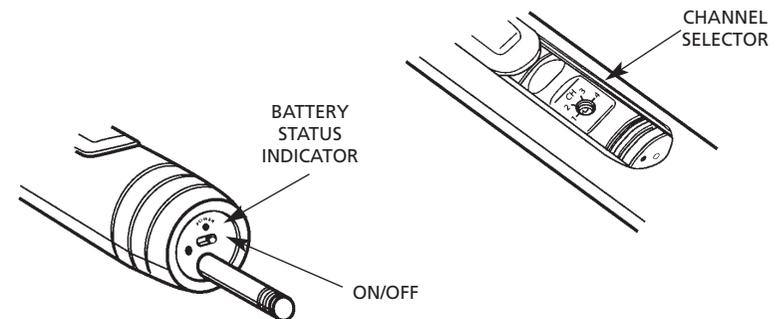
**Note:** The Transmitter only changes Active Channel when turned **off** and then **on**.
