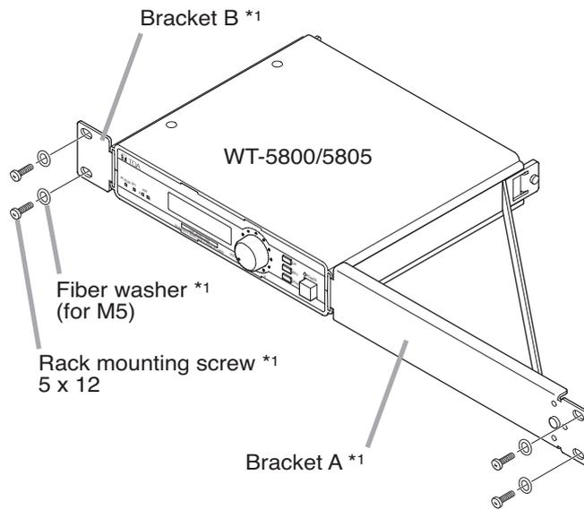
\*1 Component parts of the MB-WT3.
