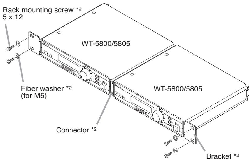
\*2 Component parts of the MB-WT4.
