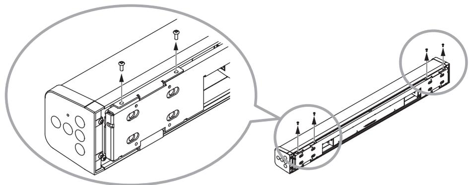
**Step 2.** Attach the wall mounting bracket to a wall. Separately prepare anchor bolts and other hardware needed for wall mounting.
