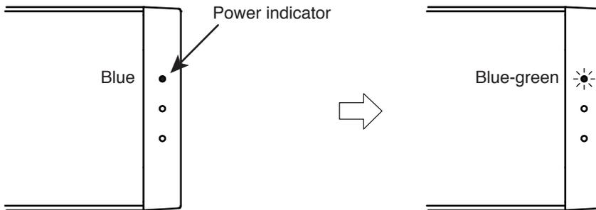
**Step 2.** Hold down the Power switch while confirming that the Power indicator is flashing blue-green.
