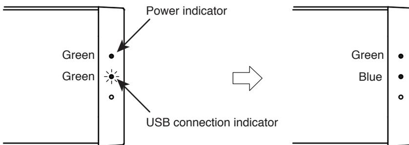
**Step 3.** After ensuring that the USB connection indicator is lit blue, release the Power switch. Initialization is complete, causing the unit to start.
