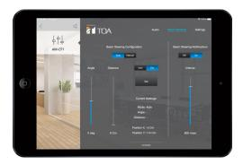
The Compass iPad must be powered on and in the Compass app to actively listen for beam steering status updates and control the KD-CamUSB
